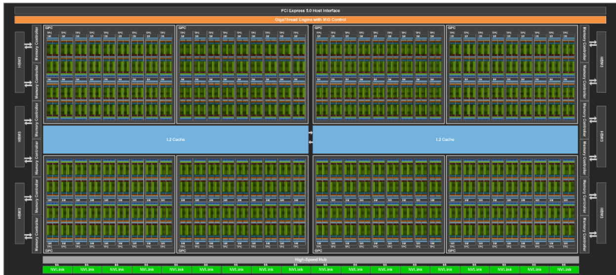
Figure 6. GH100 Full GPU with 144 SMs
